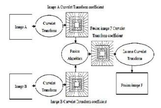
Fig. 1. Process of image fusion algorithm base on Curvelet transform.
